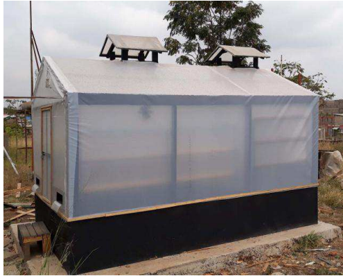
Figure 1. Experimental solar greenhouse dryer incorporated with Solid Clay- \text{CaCl}_2 desiccant energy storage system.
